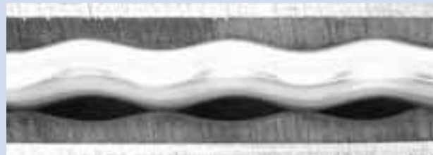
Cut-away view of the helical rotor mechanism, showing cavities that form between the rotor and the rubber stator.
